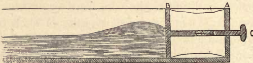
Fig. 183.—Ex.—Loop or Wave formed in Water by a Pressure at the end of a Parallel Channel.
